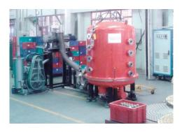
Industrial scale system to activate brass valves using plasmas for better brass rubber bonding installed in M/S Triton Valves, Mysore
